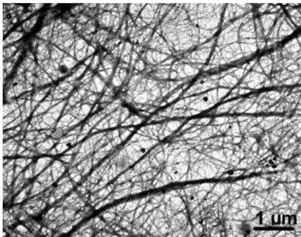
Figure 8. Transmission electron micrograph showing MFC obtained after high-pressure mechanical treatment of *Opuntia ficus-indica* fibers (SIQUEIRA *et al.*, 2010a).
