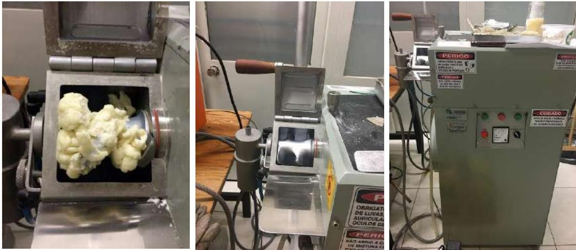
Figure 17. Photo of mixer for composite production.
