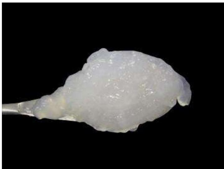
Figure 7. Picture of a 2 wt% microfibrillated cellulose aqueous suspension from eucalyptus, enzymatically pretreated (MALAININE *et al.*, 2003).
