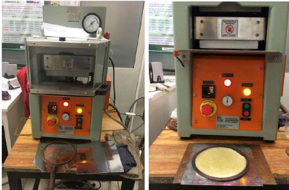
Figure 18. Compression molding equipment.
