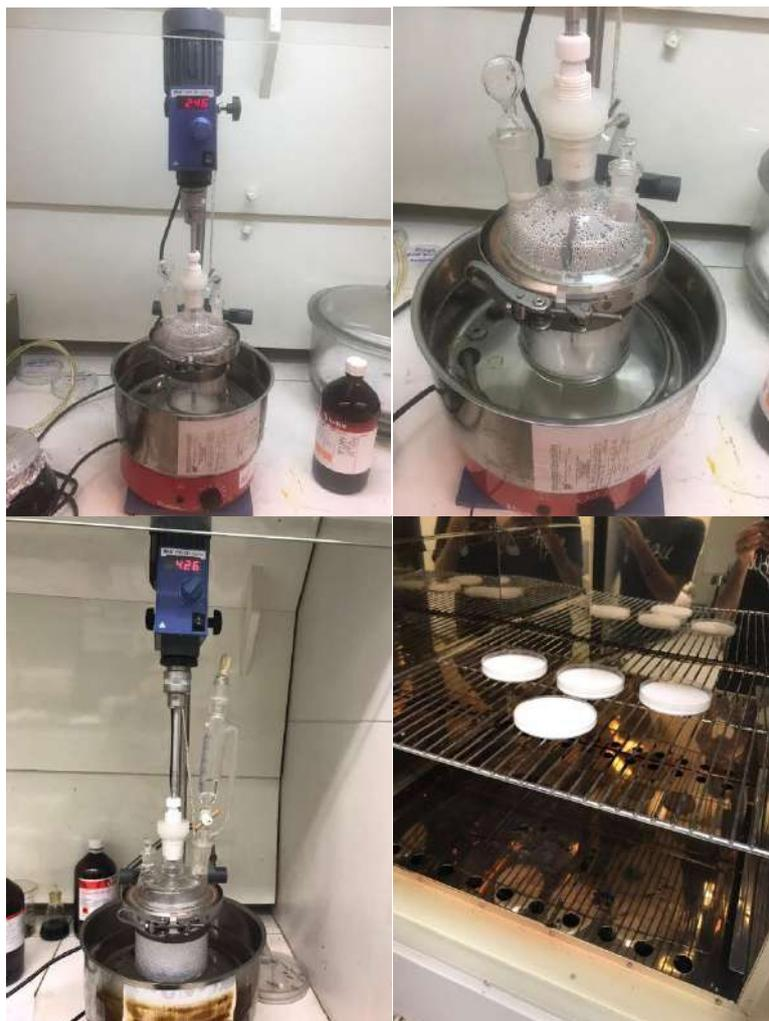
Figure 20. Reactor of preparing the gelatinized starch and SNP.
