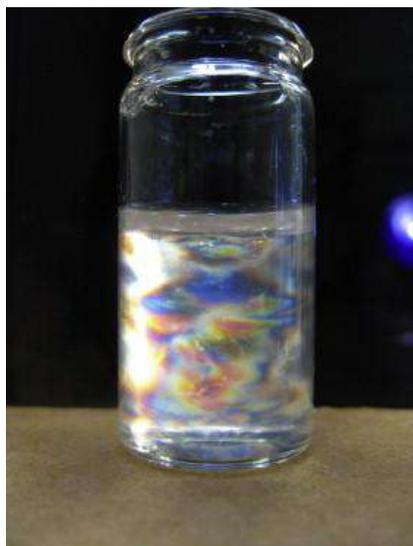
Figure 9. Photograph of an aqueous dispersion of capim dourado cellulose nanocrystals (0.50 wt%) observed between cross-nicols showing the formation of birefringent domains (LEE *et al.*, 2009).
