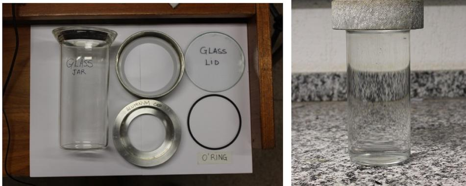
Figure 11 – Vessel components (left) and vessel assembled (right)
