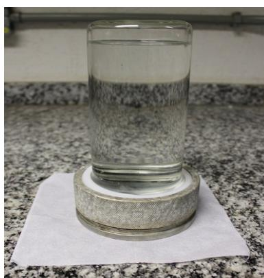
Figure 12 – Immersion vessel assembled during leakage test
