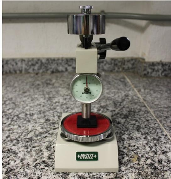
Figure 13 – Shore A hardness apparatus
