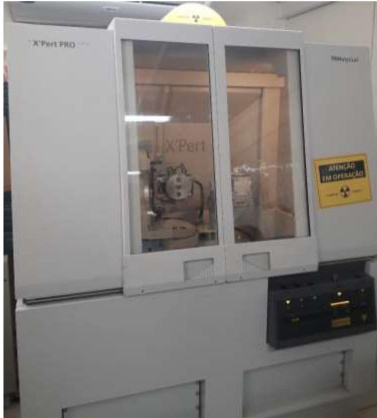
Figura 50: Difratorômetro Panalytical X'PERT PRO.
